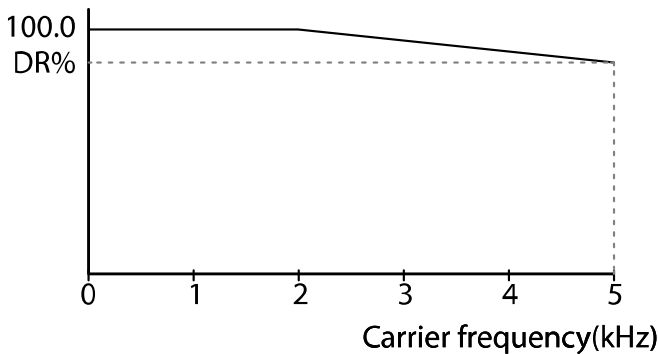
Continuous rated current for light load
